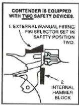
The Contender is equipped with two safety devices which function independently of each other (1. Safety position on the External Manual Firing Pin Selector. 2. Internal Hammer Block). When the Contender action is broken open properly, as explained on pages 5 and 6, the hammer block moves up into a position between the hammer and the frame. In this position the hammer cannot move forward.
